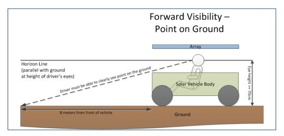
Forward Visibility – (2) A minimum of 10 degrees above the horizon on level ground.
